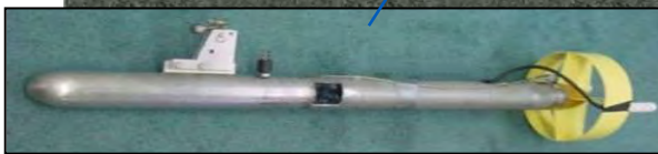
The tow fish configuration utilizes a Side Scan Sonar body retrofitted with MPM electronics, and two Ag/AgCl reference electrodes and is applicable to 550fsw / 167m.
